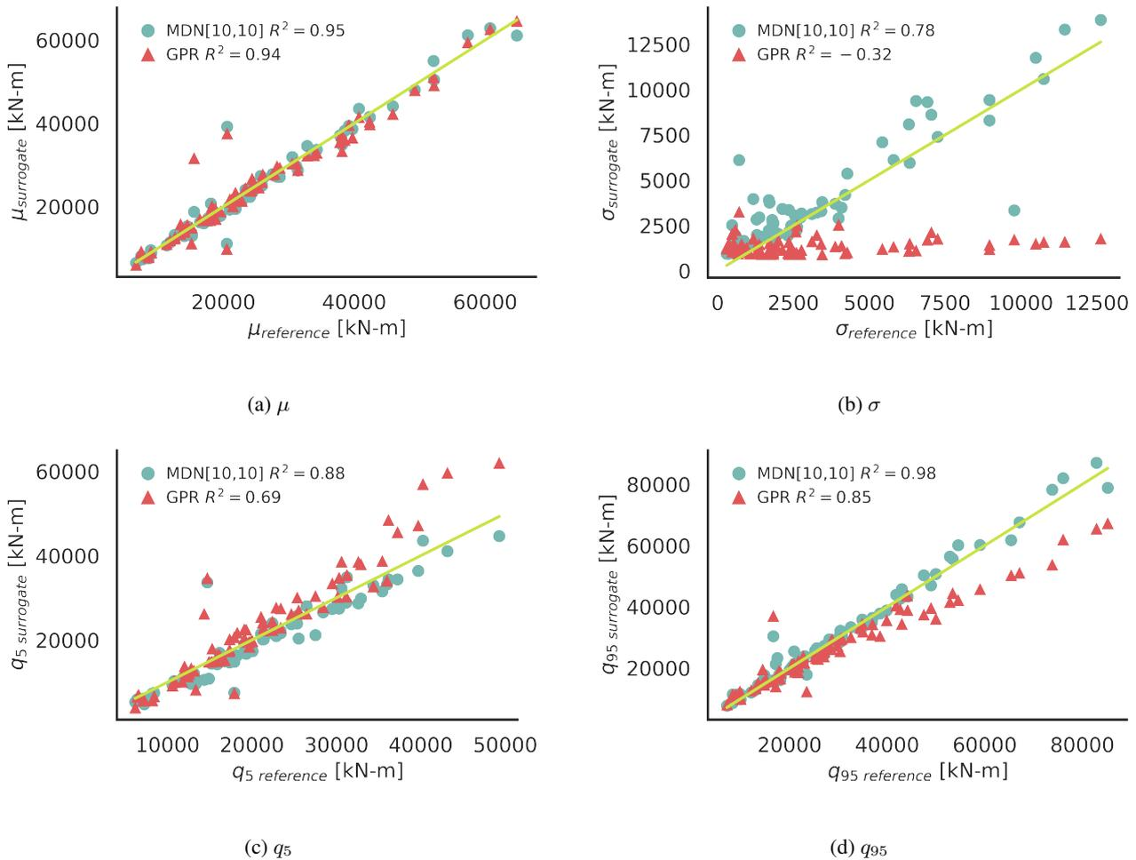
**Figure 8.** CASE-OFFSHORE: Prediction of the statistics of the response pdf of the 10-minute damage equivalent loads for the tower base fore-aft moment.
