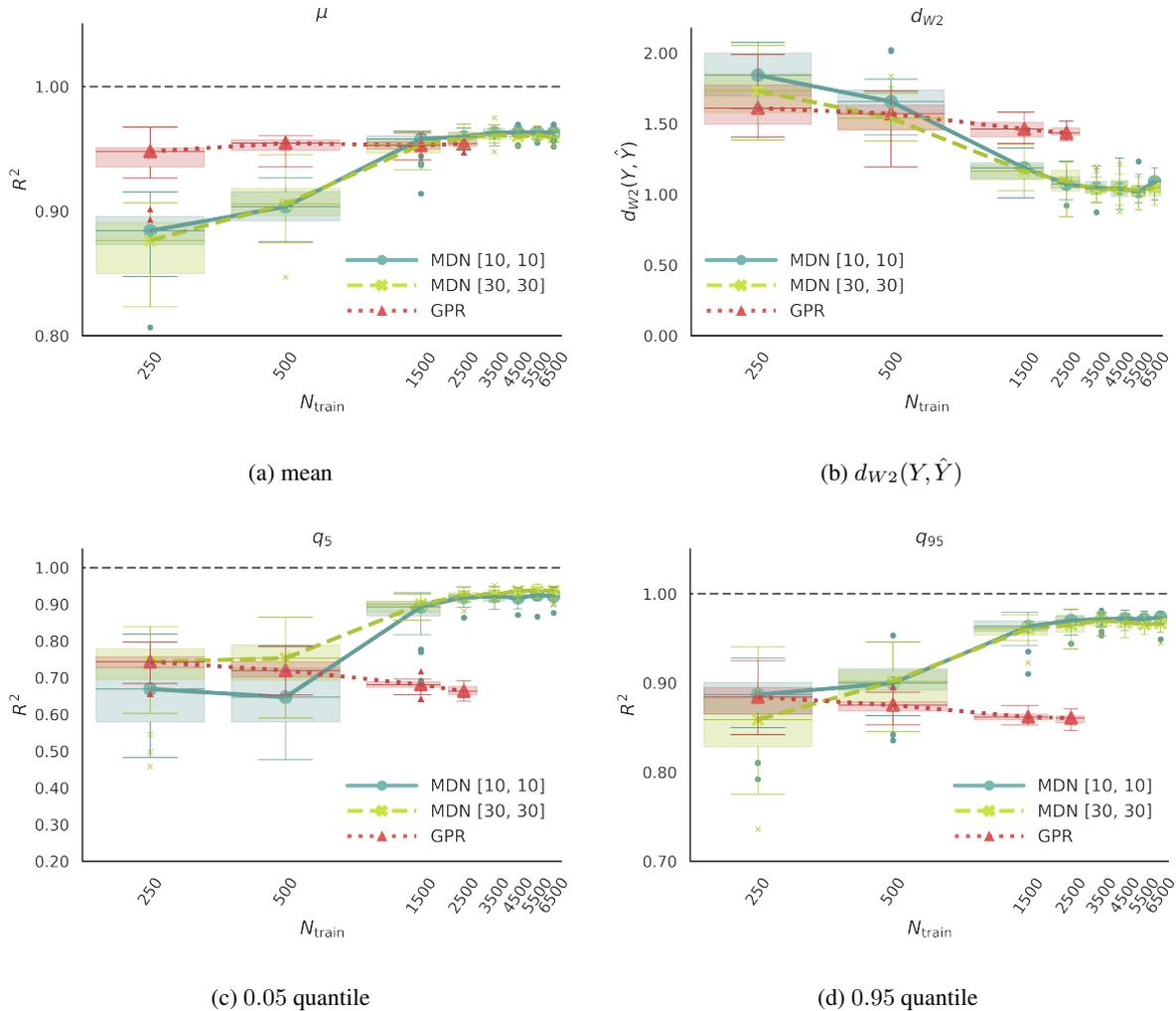
**Figure 6.** CASE-OFFSHORE: Figures showing the change in the normalized 2-Wasserstein distance,  $R^2$  value of the mean, 0.05 quantile and 0.95 quantile of the predicted pdf as a function of the training samples. The study is performed on the tower base fore-aft moment standard deviation (TwrBsMyt stddev).
