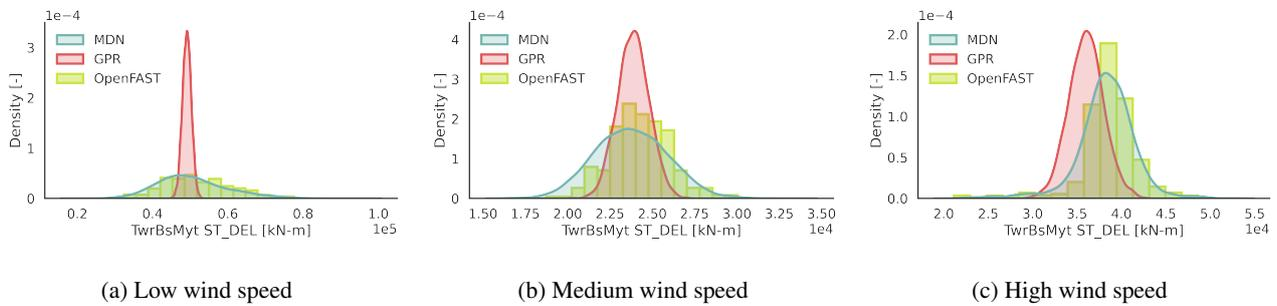
**Figure 9.** CASE-OFFSHORE: Predicted and reference (OpenFAST) conditional pdf for the tower base fore-aft moment 10-minute DEL.
