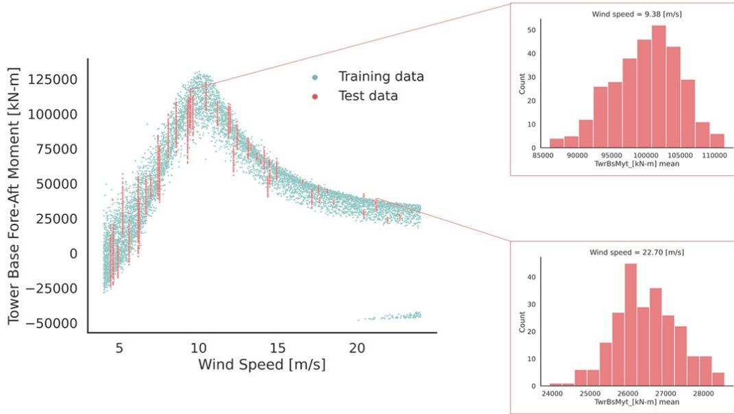
**Figure 4.** The left plot shows the 10-minute average tower bottom fore-aft moment as a function of wind speed. The samples belong to the training database of CASE-OFFSHORE. On the right, two examples of reference histograms generated using 300 turbulence seed repetitions in OpenFAST at wind speeds of  $9.38\text{ms}^{-1}$  and  $22.7\text{ms}^{-1}$  are shown from the TEST1 dataset.
