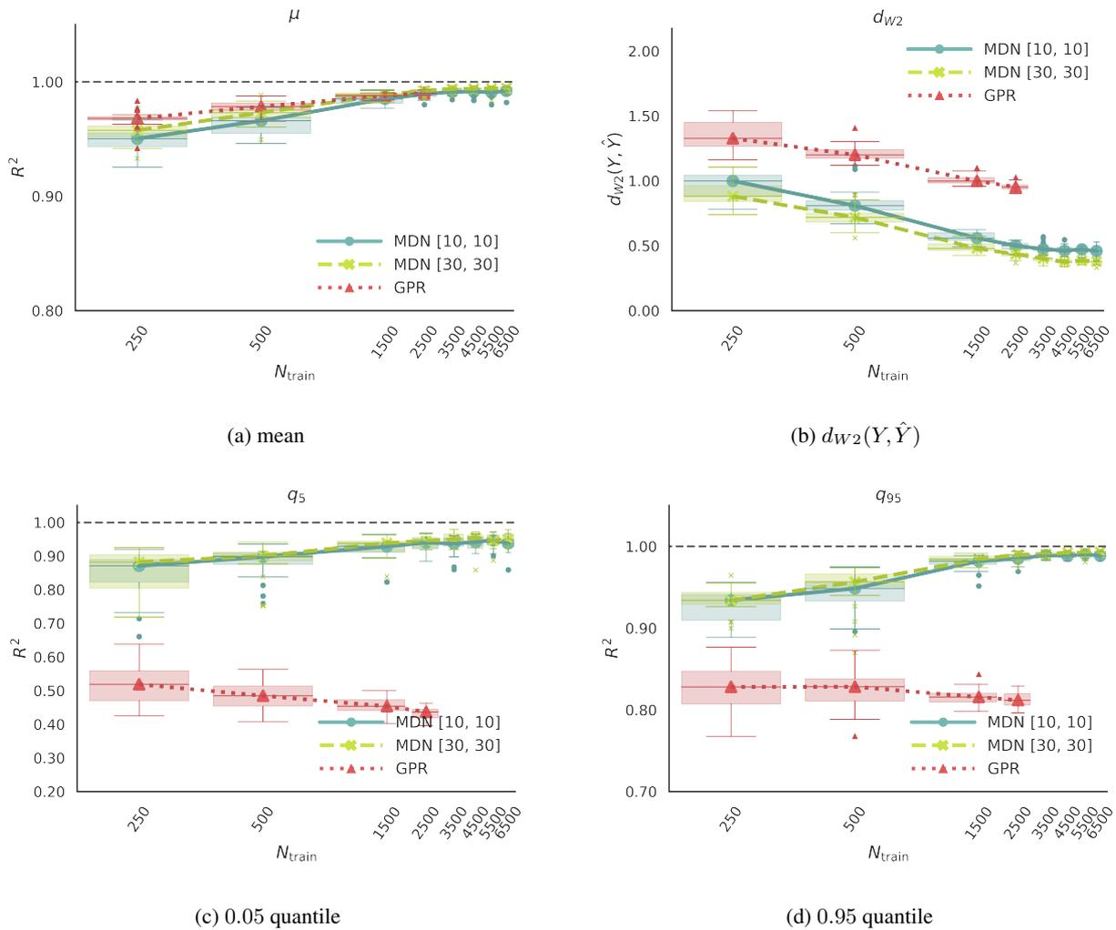
**Figure 5.** CASE-ONSHORE: Figures showing the change in the normalized 2-Wasserstein distance,  $R^2$  value of the mean, 0.05 quantile and 0.95 quantile of the predicted pdf as a function of the training samples. The study is performed on the tower base fore-aft moment standard deviation (TwrBsMyt stddev).
