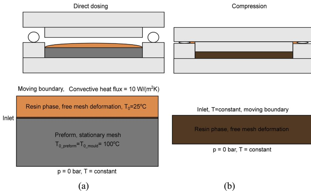
Fig. 2. Numerical domain of the models for (a) direct dosing and (b) compression with boundary and domain conditions.
