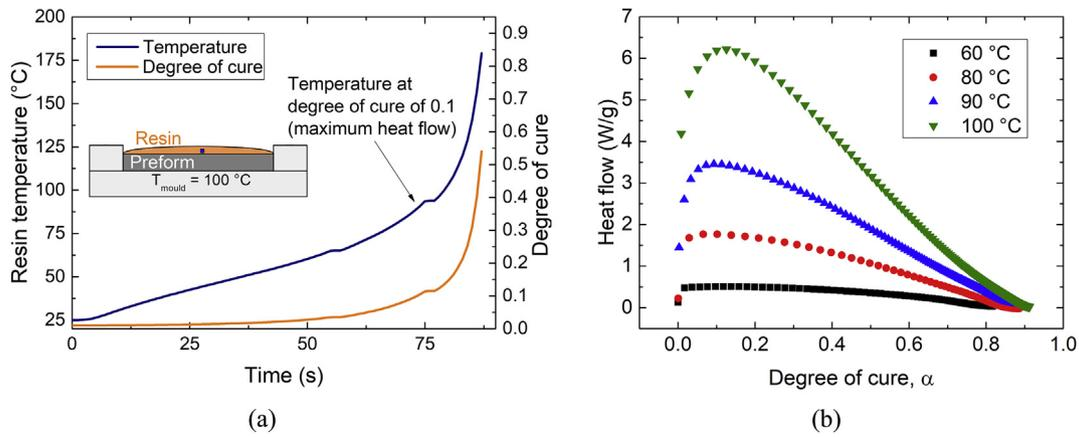
Fig. 3. Direct dosing: (a) Correlation between modelled temperature progression and degree of cure of the resin. (b) Heat flow for isothermal differential scanning calorimetry (DSC) measurements of the pure resin.
