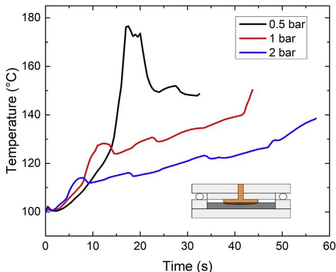
Fig. 9. Numerical results showing the maximum temperature within the resin domain during gap injection (before the compression phase) depending on the pressure, where the initial temperature of the resin and mould are 100 °C initially.
