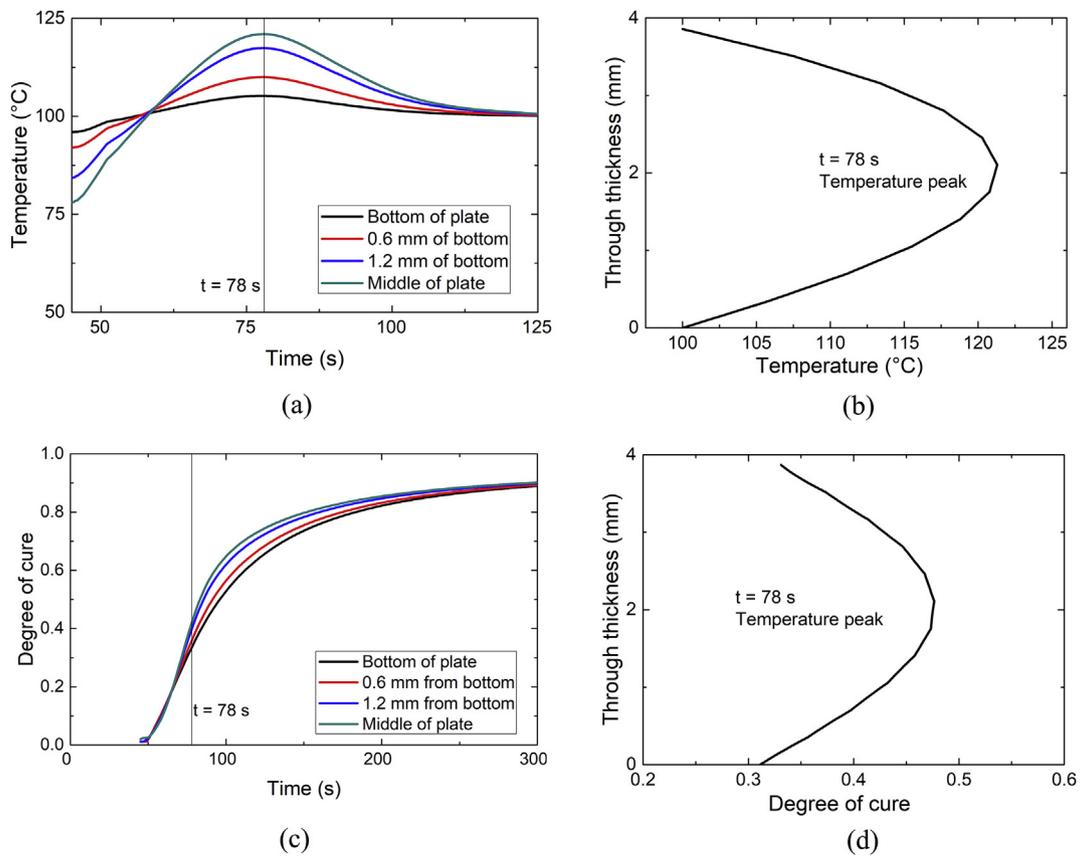
Fig. 6. Direct dosing compression stage: numerical results for (a) temperature versus time at different locations through the thickness of the composite plate, (b) temperature distribution over the thickness after 78 s (time of highest peak) (c) Degree of cure conversion at different locations through the plate thickness and (d) degree of cure distribution through the thickness after 78 s (time of highest peak) with the initial mould temperature set to 100 °C.
