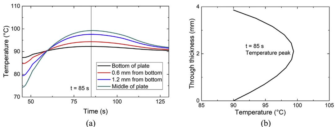
Fig. 7. Direct dosing compression stage (a) numerical temperature versus time at different locations through the thickness of the composite plate and (b) temperature distribution over the thickness after 84 s (time of highest peak) with the initial temperature at 90 °C.
