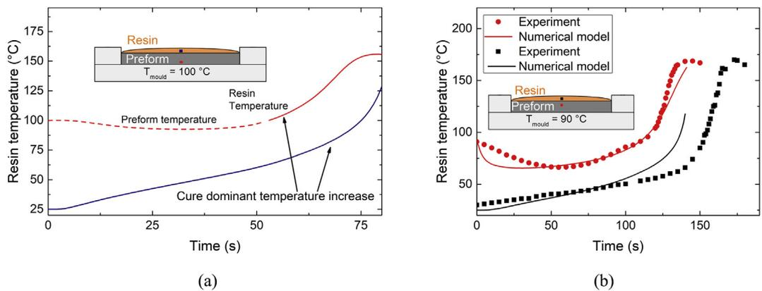
Fig. 4. Direct dosing: (a) The modelled resin temperature progression at two different locations with a mould temperature of 100 °C and (b) validation with experimentally measured values for a mould temperature of 90 °C using direct dosing.
