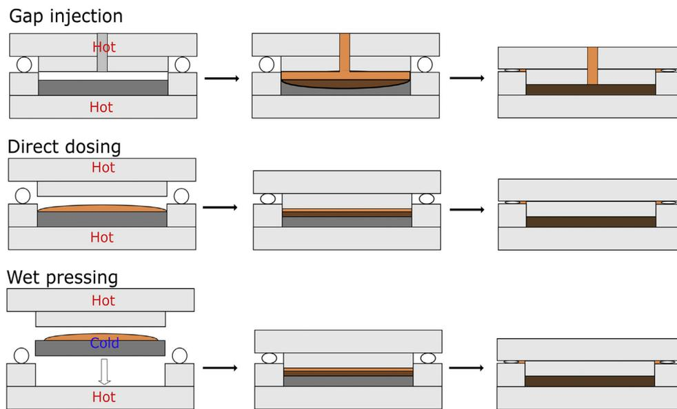
Fig. 1. Variations of the compression resin transfer moulding (CRTM) processes shown schematically.
