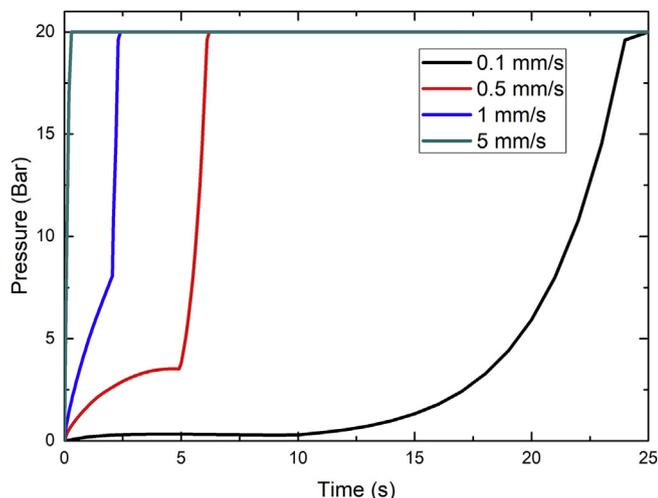
Fig. 8. Simulated pressure profile during impregnation and compaction.
