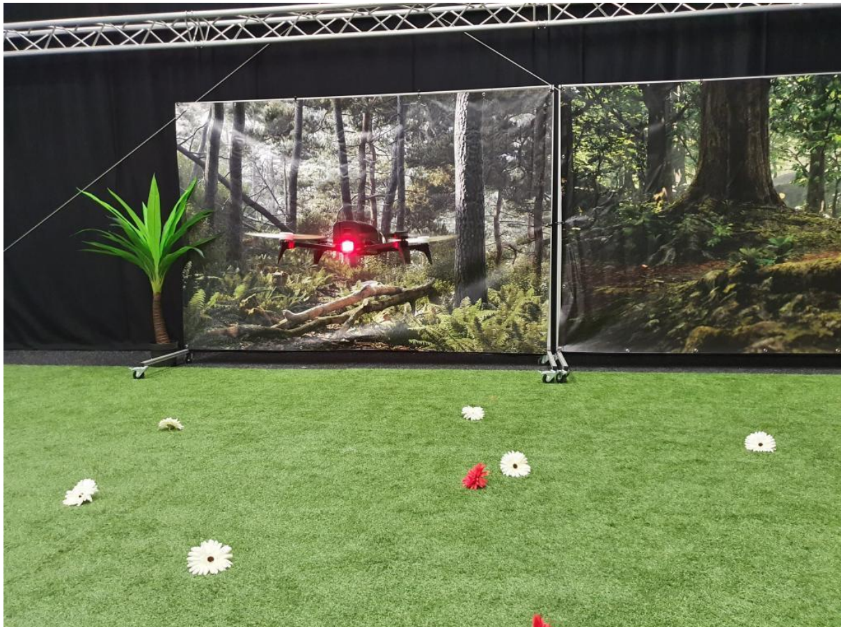
Drones can use oscillations to perceive their distance to objects. Here the drone is learning to detect and avoid obstacles in our experimental flight arena. (Image: MAVLab TU Delft)
