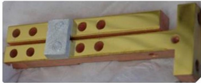
Figure 1: The extremely low contact resistance between the aluminum and copper of this heat switch was achieved by plasma etching the Al and Cu and then depositing Au without breaking vacuum [2].
