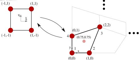
The system is solved and a global DOF vector **a** is computed. From this global vector, the nodal displacements of the element highlighted in the figure can be extracted:
