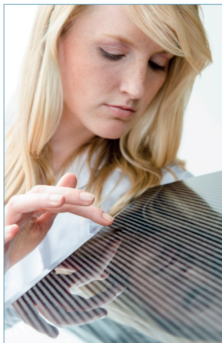
Fig. 1: Part of a convertible roof cover manufactured with a toughened, fast-cure resin
