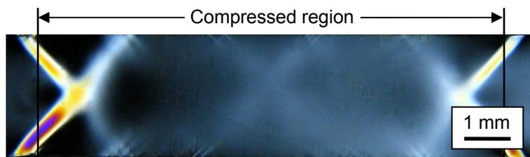
Figure 8.5. Polished section of the unmodified amine cured multifunctional epoxy shown with cross-polarised light optical microscopy.
