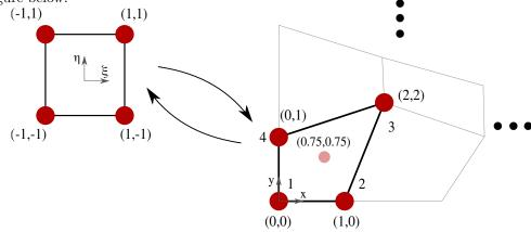
The system is solved and a global DOF vector  $\mathbf{a}$  is computed. From this global vector, the nodal displacements of the element highlighted in the figure can be extracted:
