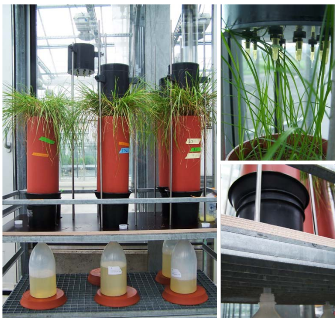
Figure 4. Microcosms and rain simulator used for the experiments. During a rain event water was drip irrigated on the grassland plants, percolated through the microcosms with a permeable bottom into a funnel and was collected in a bottle.
