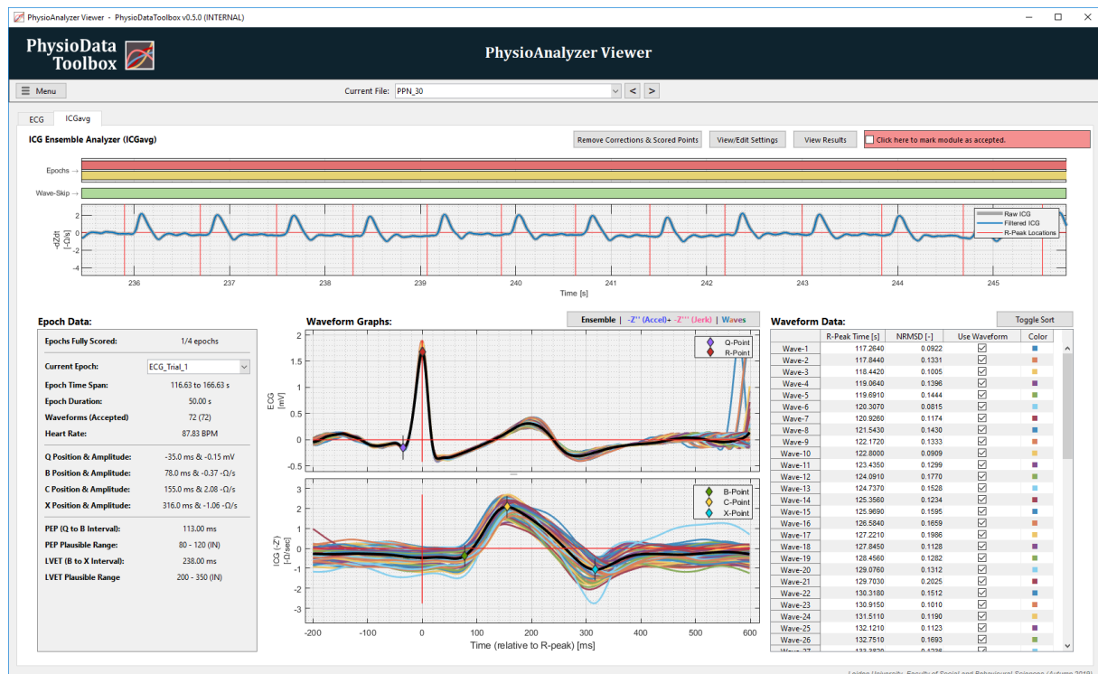
Figure 38: The ICG Ensemble Analyzer (Manual Scoring) GUI, showing: the ICG signal and the R-peak times (top graph, labeled dZ/dt); the current epoch data (leftmost table); the ensemble ECG and ICG curves, as well as the individual waveforms (two center graphs); and, the individual waveform data (rightmost table). Note that the first waveform in the table can be excluded from the ensemble by unchecking the 'Use Waveform' box. The rejected waveform is visualized by a triangle in the Wave-Skip graph, above its R-peak location.
