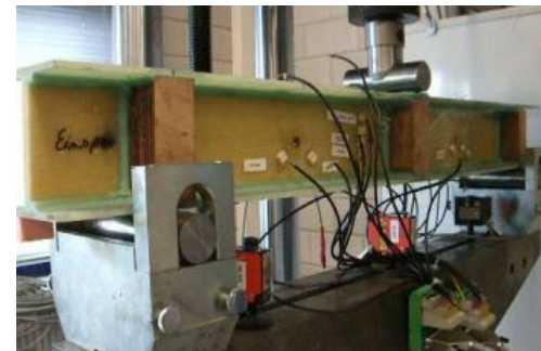
Symmetric 3pb UpWind I-beam, WMC Netherlands
