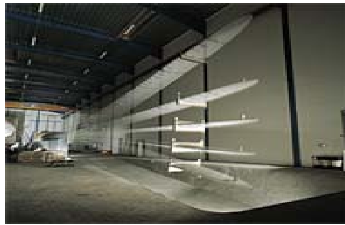
Static and fatigue tests on a single test blade
