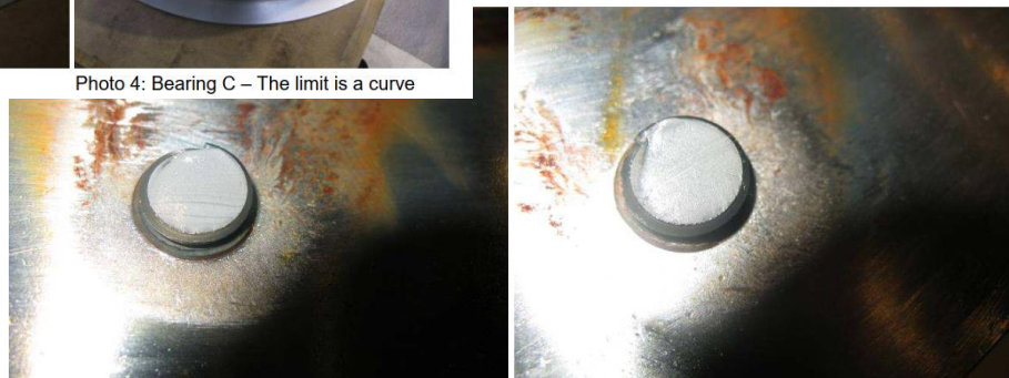
Photos 1 & 2: broken screws, part in the hub.
