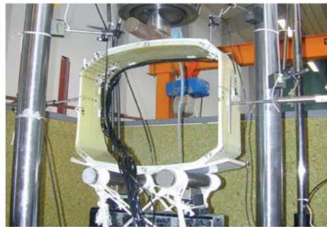
Compression of box-beam, Risoe Denmark
