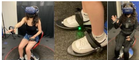
Figure 2. Locomotion via swivel chair ( left ) and shoe interface ( middle ). Right : full-body haptic suit.
