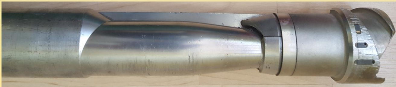
Steel shot recirculation jet bit
