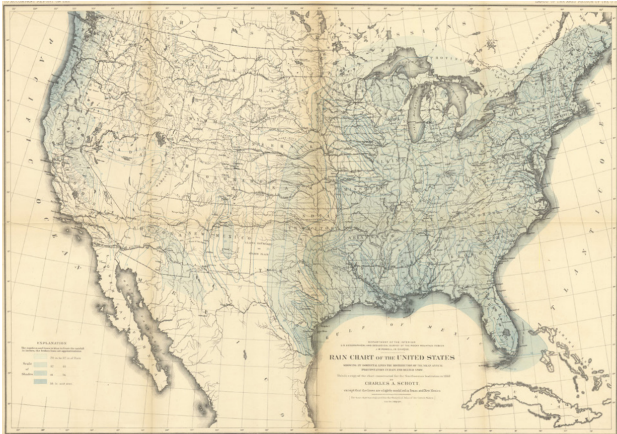
Fig 3.1 Rainfall in the United States This map by Charles A. Schott (1868) - reprinted in Powell's report - represents rainfall according to the contours of isohyet lines. The arid region is identified as the area with less than 20 inches of annual precipitation (uncoloured) which contrasts sharply with the abundant rain depicted in the East. J.W. Powell (1879), Report on the Lands of the Arid Region of the United States , Washington: Government Printing Office
