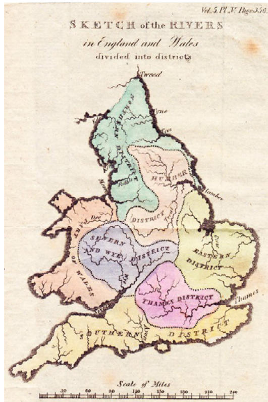
Fig 2.5 Regional constructs To the left, Dalton's geographic subdivision of England and Wales into seven districts allowed him to calculate the water balance in other catchments with reference to the hydrology of the Thames. Above, a page from a French atlas depicting the Seine's basin with its notional centre located around the economic centre of Paris.
