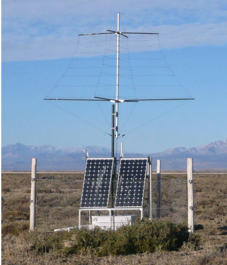
Figure 4: A radio antenna with two arms (North-South and East-West) and solar panels.[6]
