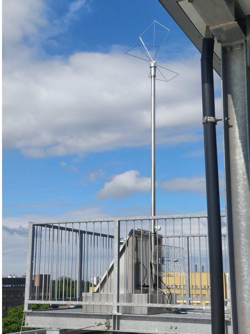
Figure 7.1: The prototype of the GRAND antenna setup installed on the roof of the Huygensgebouw (Radboud University Nijmegen). The antenna at the base is used for establishing the WiFi mesh network.
