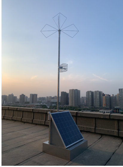
Figure 1.7: GR300 mechanical construction on top of Xidian University. The antenna, the pole the triangular box and the sandbox are visible. 9
