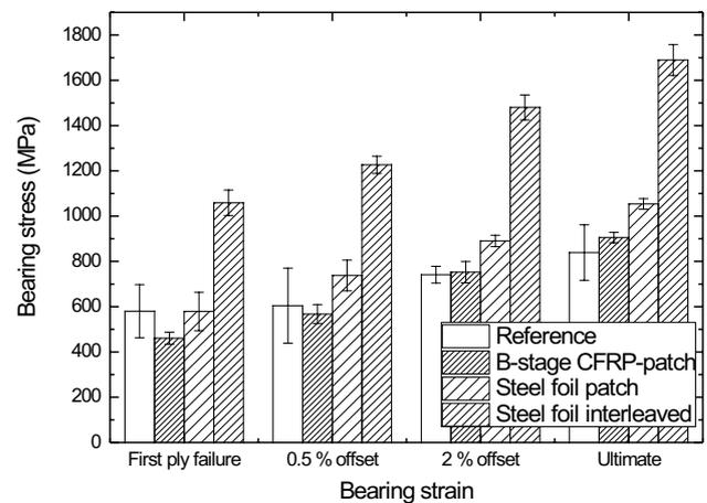
**Fig. 5** Compares the bearing stress of the reference composite, B-staged CFRP patch, steel foil patch and steel foil patch reinforcement methods at progressively increasing bearing strain offsets
