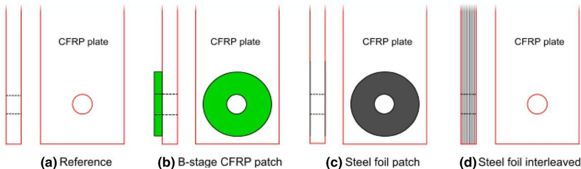
**Fig. 1** Shows the investigated local reinforcement concepts of the bearing area. **a** Reference RTM plate. **b** B-stage co-cured CFRP patch. **c** Steel foil patch around the hole. **d** Steel foil integrated in the laminate (not entire figure is shown)
