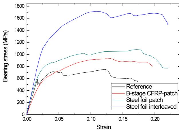
**Fig. 4** Bearing stress versus bearing strain of the locally reinforced composites in double lap bearing
