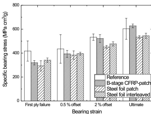
**Fig. 8** Compares the specific bearing strength of the reference composite, B-staged CFRP patch, steel foil patch and steel foil patch reinforcement methods at progressively increasing bearing strain offsets
