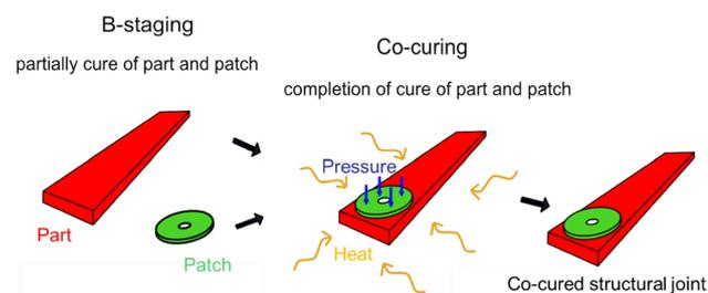
**Fig. 2** Shows the concept of local patch reinforcement of a structural part via co-curing of B-stage cured components
