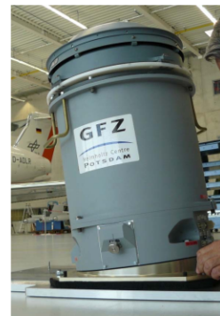
GFZ's airborne gravimeter on HALO: CHEKAN - AM
