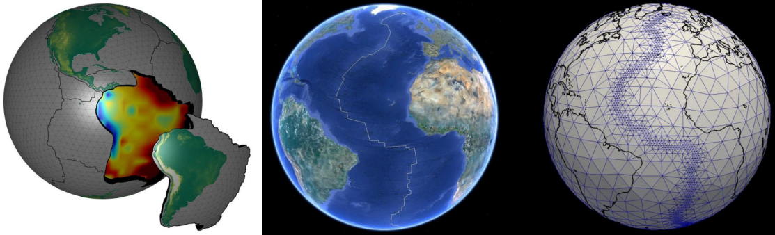
Left: Grid of a global neo-tectonic SHELLS model coupled to a global mantle circulation model; colours represent temperatures (red=hot, blue=cold) at a depth of 200km below the surface. Taken from Oeser et al. (2009) [1009]. Right: Taken from the GeoTess software 13 manual.
