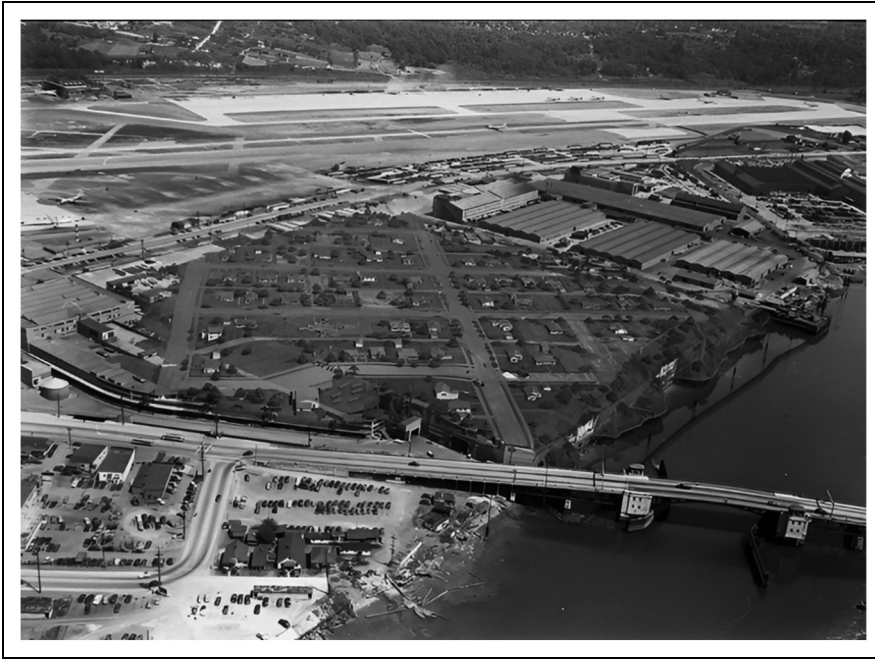
Figure 5. An aerial view of Boeing plant 2 in Seattle, nicknamed “Boeing wonderland” due to its elaborate camouflage. The photograph clearly shows the “street grid” of the sprawling faux suburb that covered the factory. Figure from Warfare History Network (2013).
