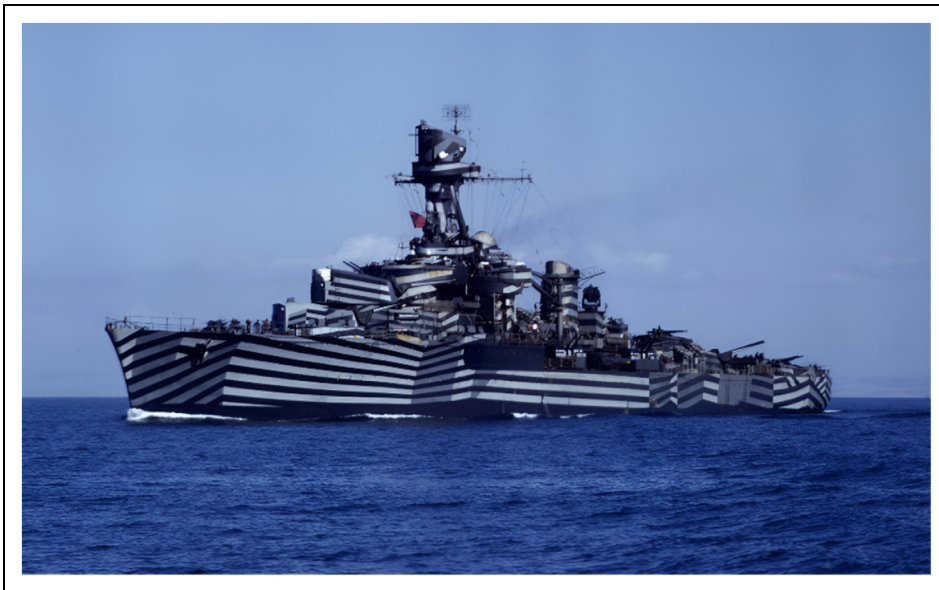
Figure 2. The French cruiser Gloire, probably during exercises off Africa, 1943/1944. Note how the dazzle pattern obscures the direction in which the bow faces. U.S. Navy photo 80-G-K-1208.
